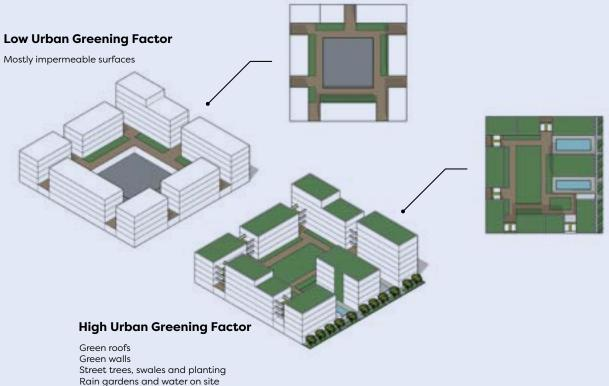
FIGURE 24: APPLYING THE URBAN GREENING FACTOR TO MAKE AN APARTMENT SCHEME MORE PERMEABLE FOR WATER
